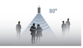
Minimum lateral sound radiation and a short distance allows focused acoustic irradiation to the visitors.
